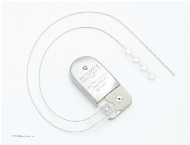
Fig. 9 An implantable part of the RNS System is comprised of a neurostimulator and depth and/or subdural cortical leads. The neurostimulator connects one or two leads placed surgically at the seizure focus. Courtesy of NeuroPace, Inc.
