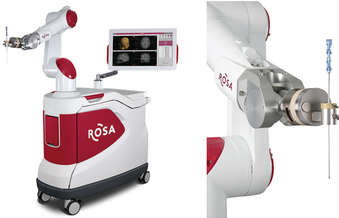
Fig. 4 ROSA, a neurosurgical robot is useful for frameless implantation of depth electrodes for SEEG. In addition, this robot has been utilized for other neurosurgical procedures such as neuroendoscopy, stereotactic biopsy, pallidotomy, shunt placement, DBS procedures, and stereotactic cyst aspiration. Courtesy of Zimmer Biomet, Warsaw, IN, USA, 2020. DBS: deep brain stimulation, SEEG: stereotactic electroencephalography.
