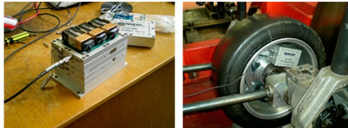
Figure 4. SoMat ® 2000 installed in the tire.
