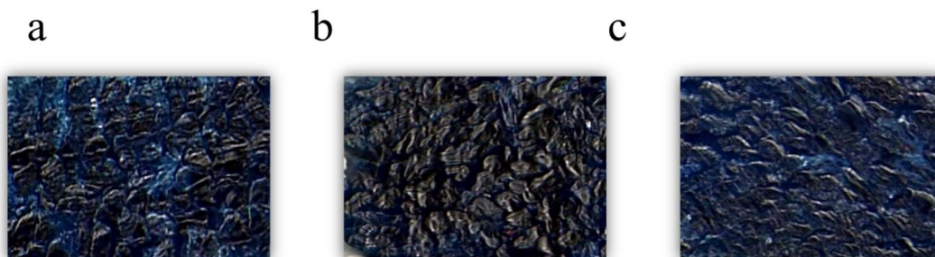
Fig. 12 Fabrics cross section of (a) PDA-cotton, (b) CHPTAC-cotton and (c) raw cotton fabrics.
