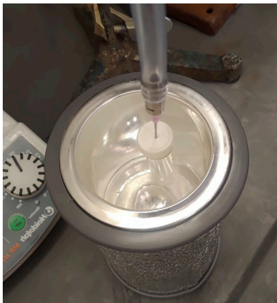
Figure 3. Freezing the reaction mixture in liquid nitrogen
