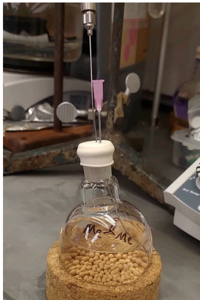
Figure 1. Solvent degassing setup
