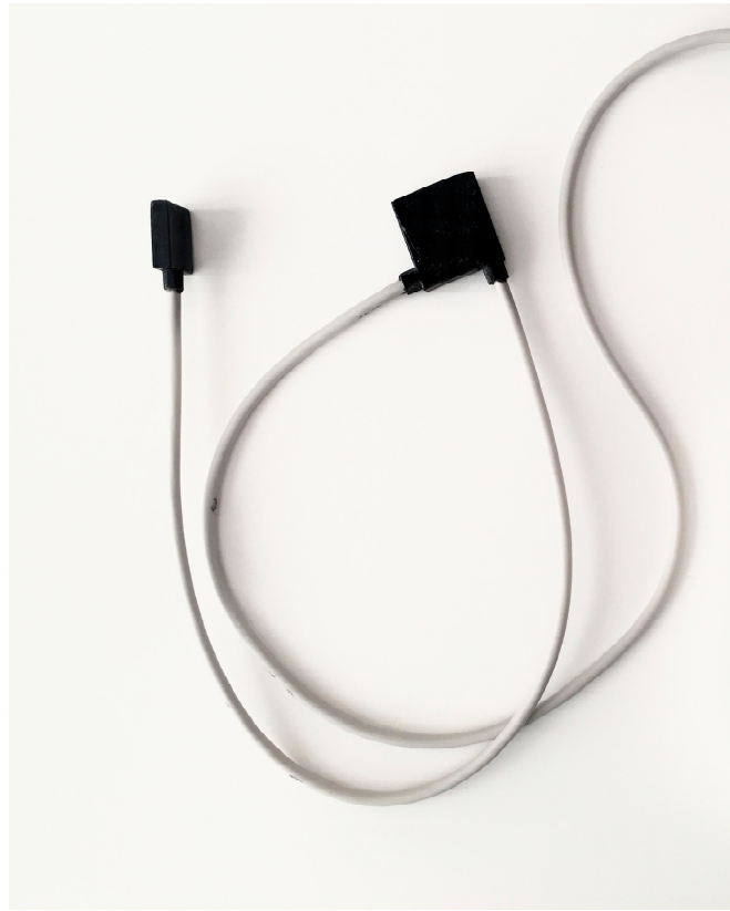
Figure 1. The system was comprised of two sensor units, one of which was larger and acted as a master unit synchronising the sensor data. The units were connected via a cable.
