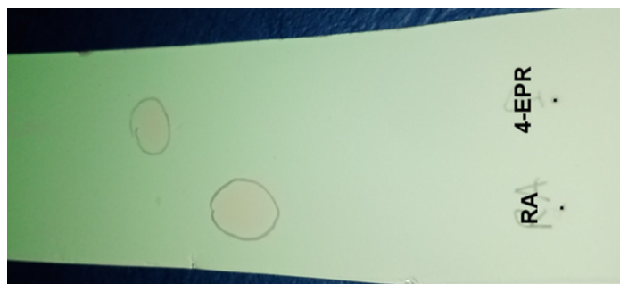
Figure 2. TLC profile of ATRA (in the image RA, R_f = 0.45 ) and of 4-EPR ( R_f = 0.61 ).
