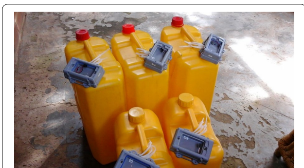
Fig. 1 GPS-enabled jerry cans (20 and 10 L) with batteries awaiting installation
