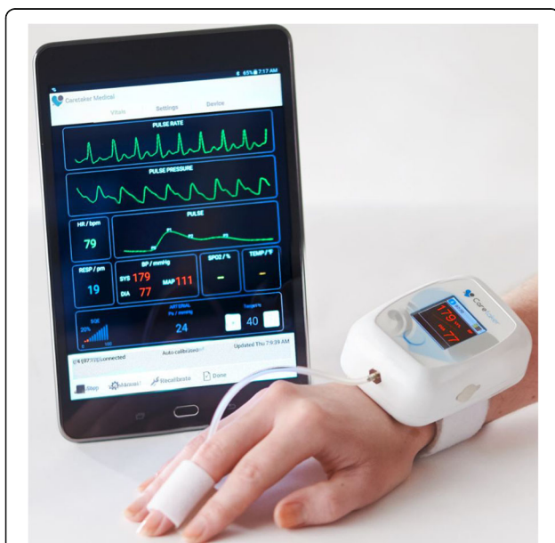
Fig. 1 CareTaker Wireless Continuous Blood Pressure and Heart Rate Monitor with Finger Cuff Technology. Copyright 2016. Used with written permission from president and CEO of CareTaker Medical, LLC
