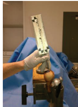
FIGURE 3: Right humerus. MicronTracker 2 H3-60 three-dimensional optical tracker (Claron Technology Inc., Toronto, Ontario) mapping out the contact surface area.
