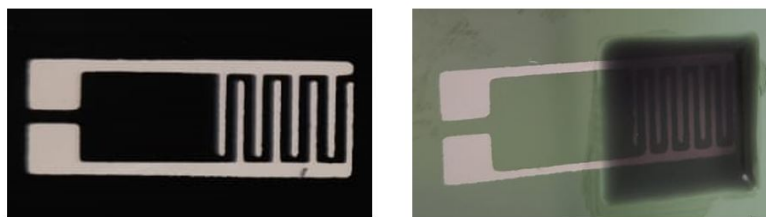
Figure 13. Screen-printed interdigital electrodes (left). CNT-PDMS composite mold-printed on top of electrodes (right). For clarification purposes a 0.2 CNT wt% solution was printed in order to leave the electrodes visible through the layer.
