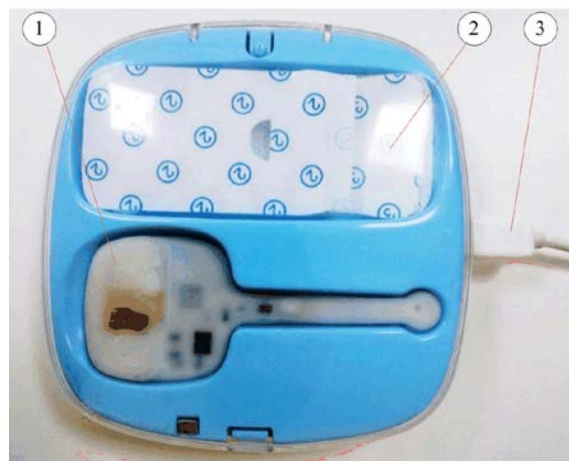
Figure 12. The developed smart thermometer product: (1) the Bluetooth thermometer, (2) the monitor screen, and (3) an extra charging port.
