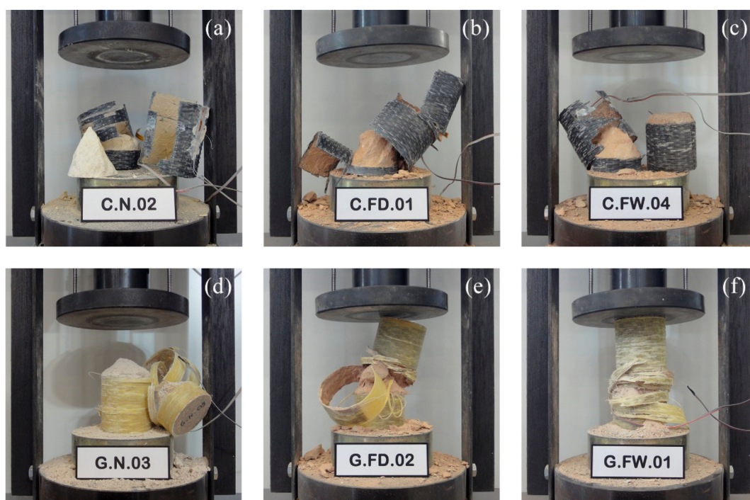
Figure 8. Examples of failure of FRP confined stone samples: CFRP, (a) undamaged, or after fire exposure with (b) slow air-cooling or (c) quick water-cooling; GFRP, (d) undamaged, or after fire exposure with (e) slow air-cooling or (f) quick water-cooling.
