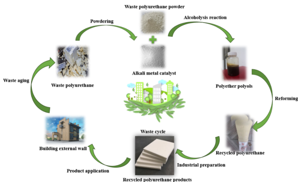
Figure 4. Schematic diagram of the green recycling process of degrading waste PIR.
