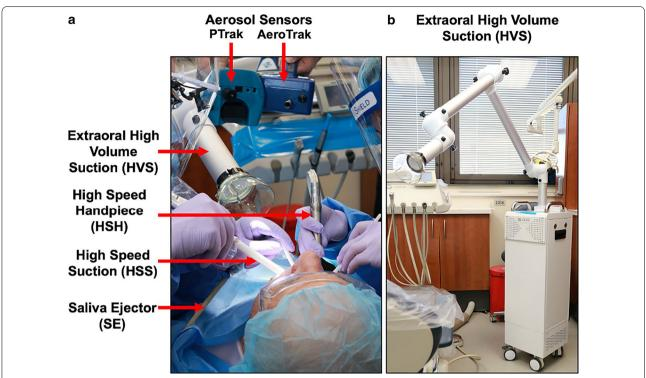
**Fig. 1** Experimental setup for the dental procedures and aerosol measurements. **a** Locations of the different suction systems including saliva ejector (SE), high speed suction (HSS) and extraoral high volume suction (HVS). Locations of the aerosol meters during data acquisition. **b** The HVS device use for the experiment
