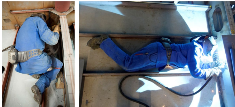
Fig. 1 Shipyard welders in non-neutral positions (Image source: used by courtesy of MEYER WERFT GmbH & Co. KG.)
