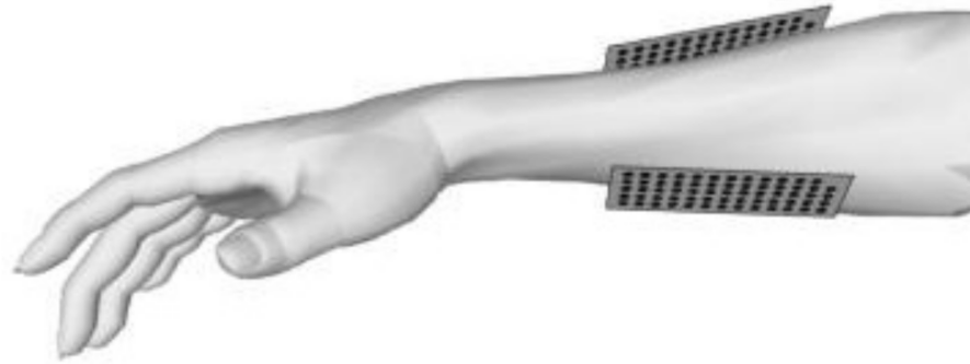
Fig 1. The placement of the high-density EMG sensors in the finger movement experiment.
