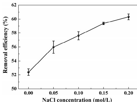
**Figure 10.** Influence of ionic strength on the removal amount of MB (dosage of the adsorbents: 1.0 g/L; initial concentration: 200 mg/L).
