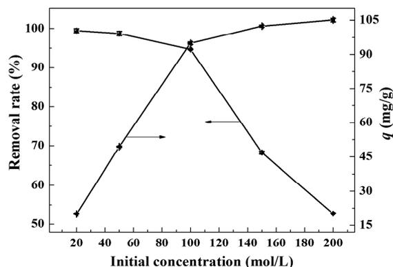
**Figure 11.** Effect of initial concentration on the MB adsorption (dosage of the adsorbents: 1.0 g/L).
