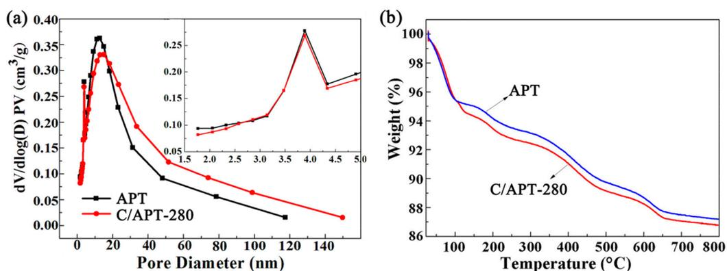
**Figure 2.** (a) Pore size distributions of APT and C/APT-280; and (b) TG curves of APT and C/APT-280 under an oxygen atmosphere.
