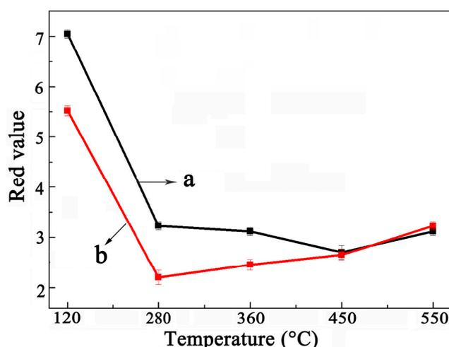
**Figure 3.** Change of red values of crude palm oil after being decolorized by the APT (a) and C/APT (b) calcined at different temperatures (SD,  $n = 6$ ).
