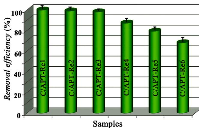
**Figure 12.** The removal efficiency of the re-generated C/APT-Re adsorbent for MB (dosage of the adsorbents: 2.0 g/L).
