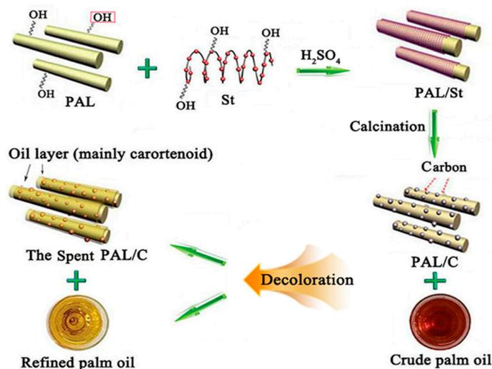
**Scheme 1.** A schematic diagram of the preparation and decoloring procedure.
