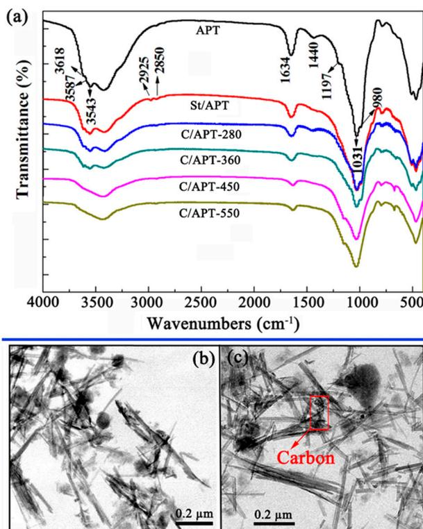
**Figure 1.** FTIR spectra of APT, St/APT precursor and the C/APT adsorbents prepared at different temperatures (a); and TEM images of APT (b) and C/APT-280 (c).
