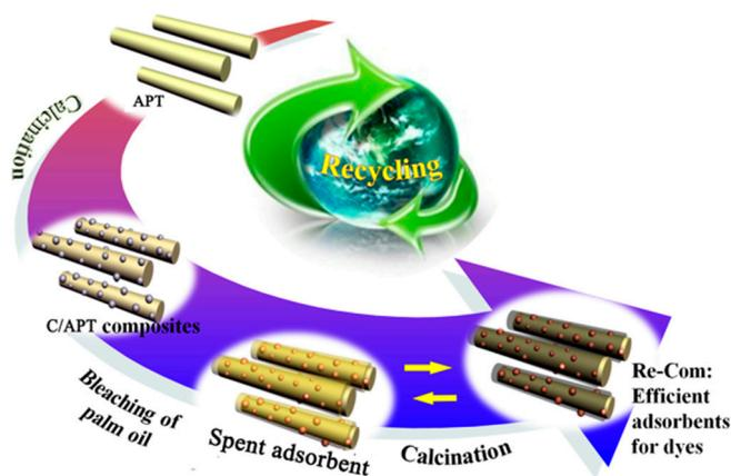
**Figure 13.** The cyclic regeneration and reusable route of C/APT decolorant, spent decolorant, and dye-loaded adsorbent.
