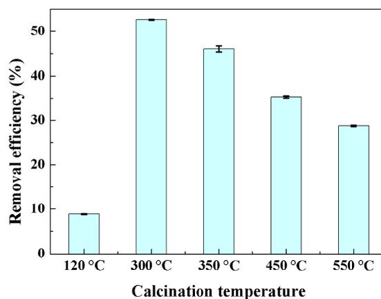
**Figure 8.** Effects of calcinations temperature on the adsorption efficiency of the used adsorbent (adsorbent dosage: 1.0 g/L).
