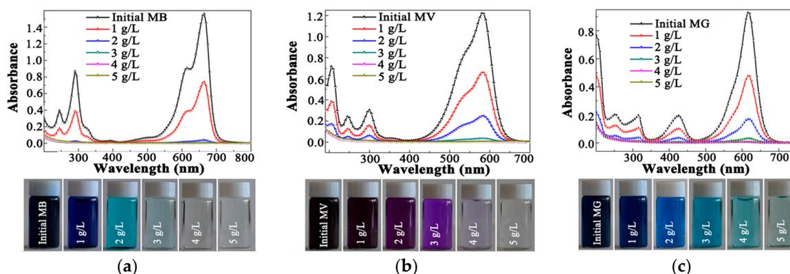
**Figure 7.** UV-VIS spectra of MB (a), MV (b), and MG solutions (c) after adsorption by C/APT-Re1; digital photographs of the MB, MV, and MG solutions.
