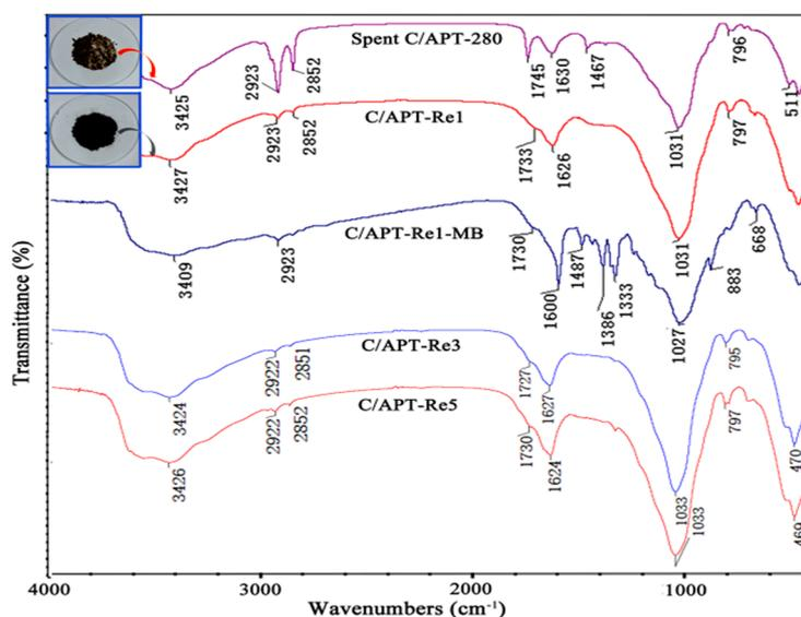
**Figure 4.** FTIR spectra of the spent C/APT-280 decolorant, C/APT-Re1 and C/APT-Re1-MB, C/APT-Re3 and C/APT-Re5. The inset shows digital photographs of spent C/APT-280 and C/APT-Re1, respectively.
