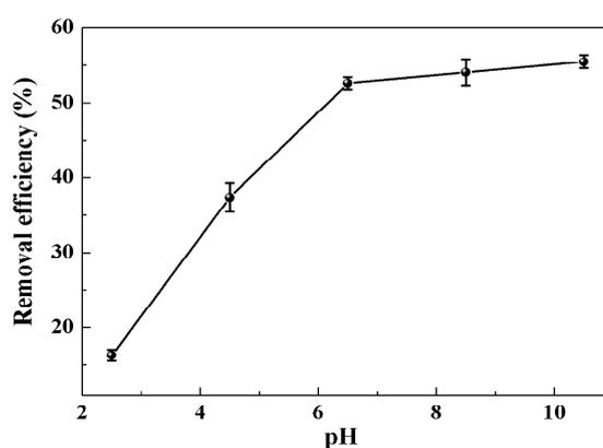
**Figure 9.** Effect of pH on the removal rate of MB (dosage of the adsorbents: 1.0 g/L; initial concentration: 200 mg/L).
