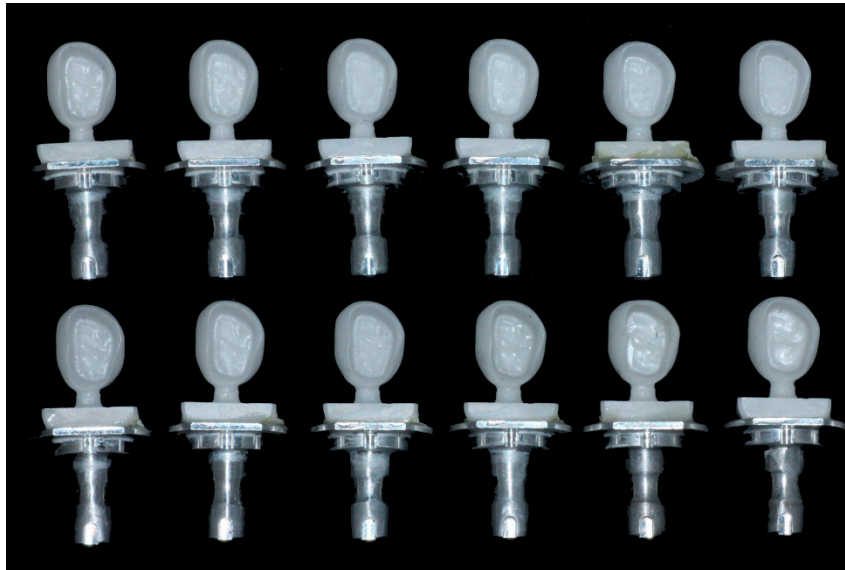
Figure 2. Monolithic zirconia crowns fabricated by milling fully sintered (Y,Nb)-TZP blocks in a chairside computer-aided design–computer-aided manufacturing (CAD–CAM) system for single-visit dentistry.
