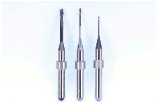
Figure 3. Milling tools used for partially sintered 3Y-TZP blocks: \Phi 2.0 mm (left), \Phi 1.0 mm (middle), and \Phi 0.6 mm (right).
