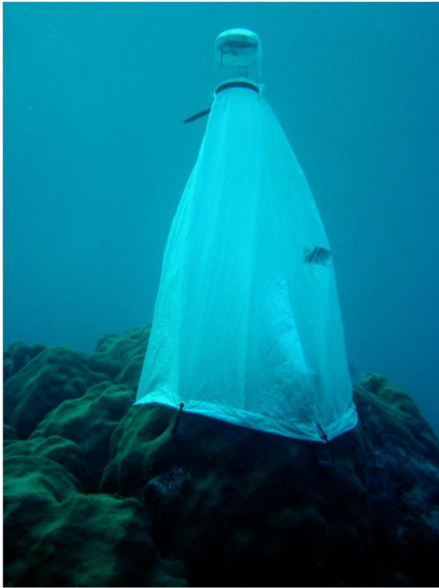
Figure 1. Spawning tent used to collect gametes from coral colonies. Photo: Erich Bartels. doi:10.1371/journal.pone.0010898.g001
