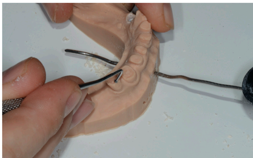
Figure 7. The tracer tool slides above the teeth for a 15 cm path to perform the required accuracy check.
