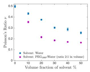
**Figure 5.** Evolution of the Poisson ratio of hydrogels fabricated from different photosensitive solutions as a function of the solvent volume fraction. Two different solvents are shown: water (blue markers) and a solution of PEG  $M_n = 1000$  g/mol:water at a volume ratio of 2:1 (purple markers).
