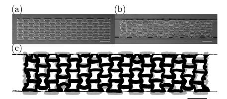
**Figure 6.** Auxetic metamaterial fabricated from a solution of 90% PEG-DA  $M_n = 700$  g/mol and 10% photo-initiator in volume. (a) Before compression, (b) submitted to an uniaxial compression, (c) superposition of the undeformed and deformed shapes. The particle width and length decreased when compressed, which is indicative of a negative Poisson's ratio.
