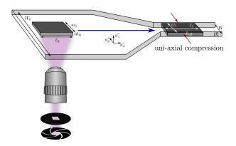
**Figure 1.** In situ fabrication of a particle using a microscope-based projection lithography technique. UV light is projected into a flat channel through a shutter and a rectangular mask resulting in the fabrication of a hydrogel particle surrounded by uncured solution. The slab is then pushed into a constriction by applying an external flow. When the particle has completely entered the narrow region of the channel the flow is stopped and the particle experiences uni-axial compression.
