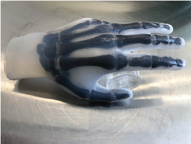
Fig. 1. A fully assembled model is visualized, with the radiopaque bones visible through the dorsum. A thicker consistency silicone was utilized for the base, whereas a less viscous silicone, which is more translucent and allowed greater flexibility, is used on the dorsum.
