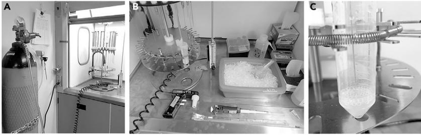
**Figure 1. Purging O<sub>2</sub> from the gelation solution**
