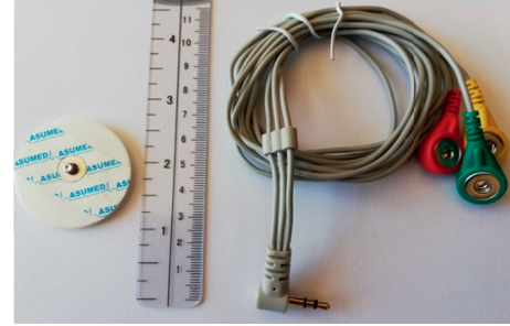
FIGURE 2: Example view of electrodes and shielded cables.
