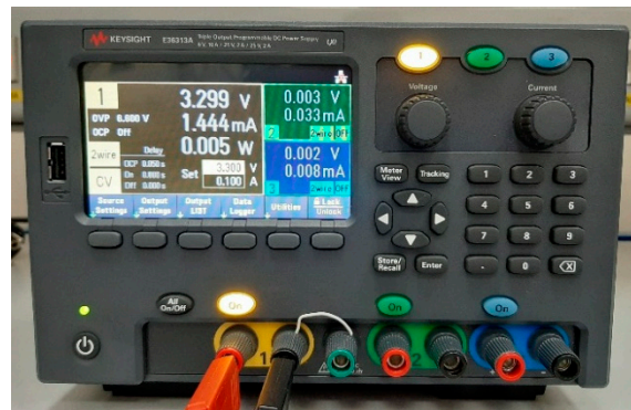
Figure 9. Power supply of the low-power analog front end, measuring the current drawn by the circuit.
