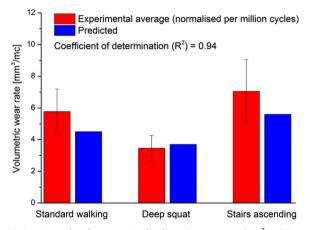
Fig. 11. Experimental and computational volumetric wear rates  $[mm^3/mc]$  (mean  $\pm$  95% CI, n = 6) under standard walking, deep squat, and stairs ascending kinematic conditions.
