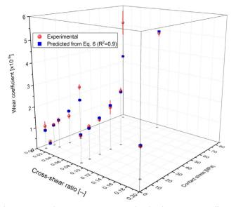
Fig. 9. Experimental (mean  $\pm$  95% Cl, n = 6) and predicted (Eq. (6)) wear coefficients for moderately cross-linked UHMWPE under different cross-shear ratios and different contact stresses.
