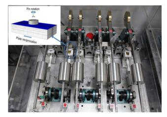
Fig. 2. Multidirectional pin-on-plate wear simulator.
