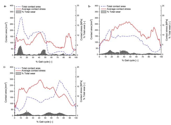
Fig. 10. Predicted contact area [mm<sup>2</sup>], average contact stress [MPa], and percentage contribution to the total wear at different percentage of the loading cycle under standard (a), deep squat (b), and stairs ascending (c) kinematic conditions.
