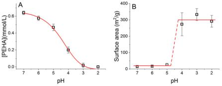
**Figure 6: Representative property changes upon acidification of coagulated silica material.** (a) Change of additive concentration with respect to pH, and (b) change of silica porosity with respect to pH. Reproduced from Manning *et al.* <sup>13</sup> under Creative Commons license.
