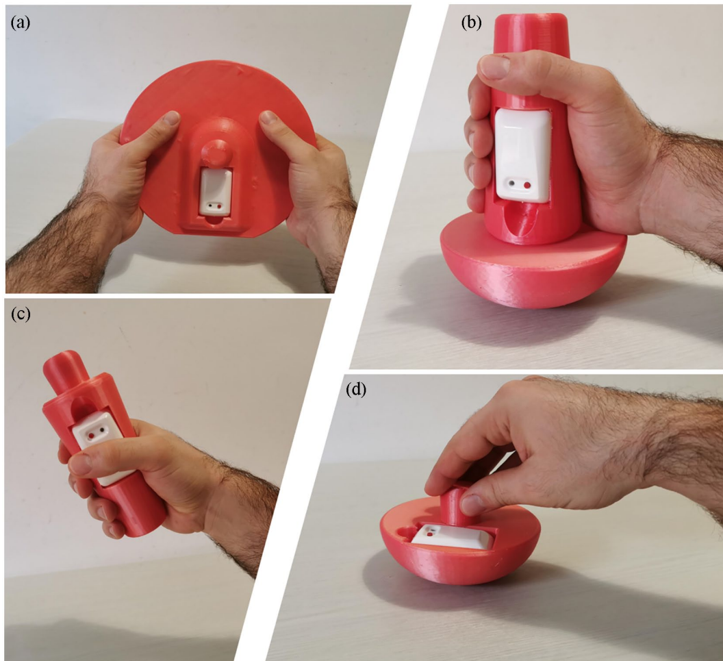
Figure 1. Smart object, three-dimensional objects printed in plastic material: (a) the disc is used to perform coordinated and specular movements of prono-supination of the wrists, (b) the joystick is used to perform shoulder flexion, elbow flexion-extension and ipsilateral prone-supination movements, (c) the remote control is used to perform elbow flexion-extension, and (d) the spinning top is used to perform a correct grip of the hemiparetic hand and allow the movement of the ipsilateral upper limb.
