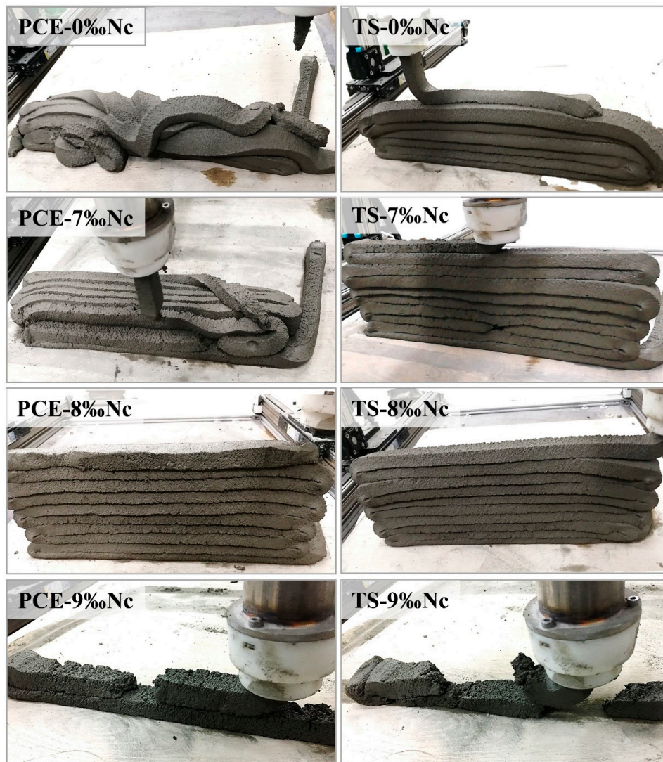
Figure 4. Demonstration of 3D printability of cement paste with different type of superplasticizers and different dosage of nano clay.
