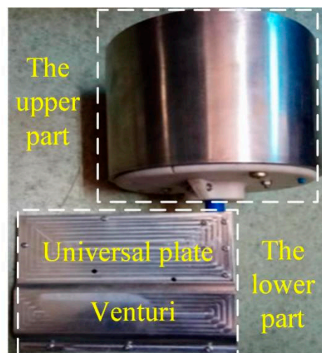
Figure 19. Sensor for monitoring flow direction and velocity.
