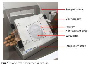
Fig. 1 Cone test experimental set-up
