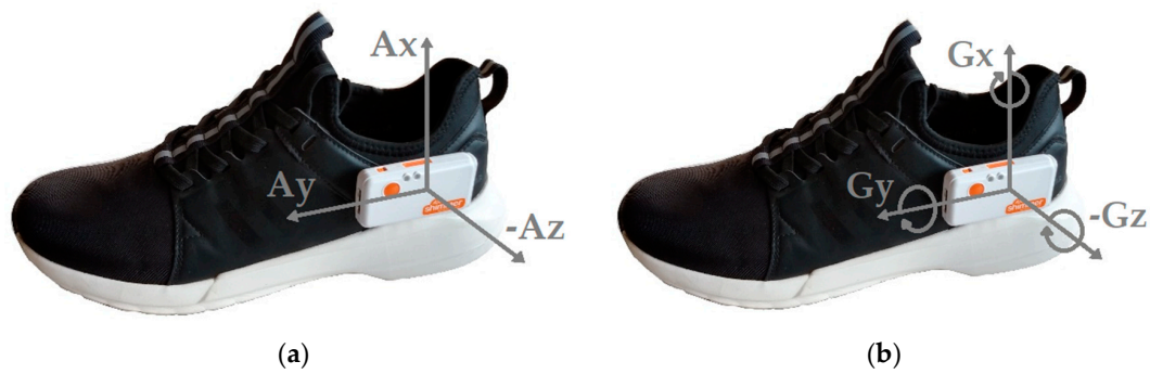
Figure 2. IMU sensor placement and axis alignment. (a) Accelerometer. (b) Gyroscope.
