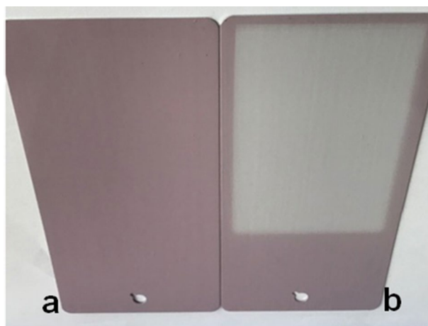
Figure 1. Colour fastness of the dye I-APU film under UV exposure (a) initial film; (b) after 414 h.
