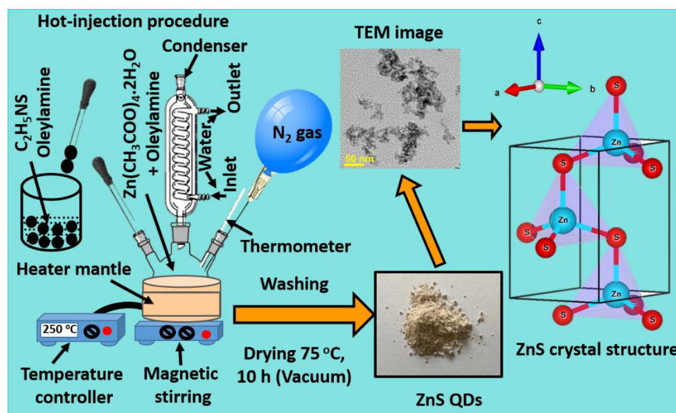
Scheme 1. Schematic representation of the ZnS quantum dots (QDs) using the hot-injection method and illustration of the crystal structure of the ZnS.
