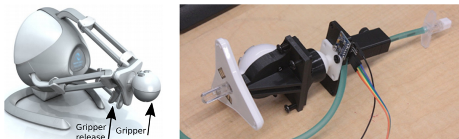
FIGURE 3: (a) Novint Falcon haptic device. (b) Custom-made (3D-printed) interface to connect the epidural needle to the haptic device.
