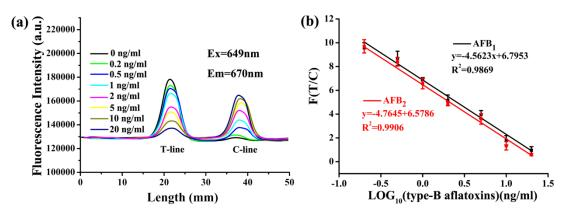
**Figure 6.** Quantitative determination of type-B aflatoxins with prepared strips. (**a**) Fluorescence spectra of T-line and C-line at different concentrations of  $AFB_1$ . (**b**) The linear relationship between the ratio of fluorescence intensity (F(T/C)) of the detection line and the control line and the logarithm of the concentration of type-B aflatoxins at different concentrations.
