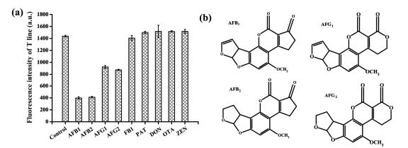
**Figure 5.** Specificity of the aptamer-based lateral flow strips (ALFs) by analyzing  $AFB_1$  against other mycotoxins at 100 ng/mL. (a) The T-line fluorescence intensity of other mycotoxins. (b) Chemical structures of  $AFB_1$ ,  $AFB_2$ , aflatoxin  $G_1$  ( $AFG_1$ ) and  $AFG_2$ .
