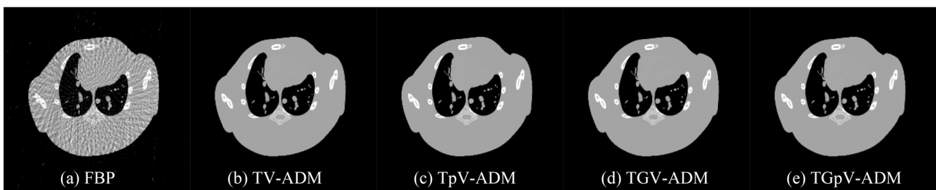
Fig 2. Image reconstruction of the Moby phantom from noise-free projection dataset. Results of the (a) FBP, (b) TV-ADM, (c) TpV-ADM, (d) TGV-ADM, and (e) TGpV-ADM minimization methods. Display window is [0.2, 1.0].
