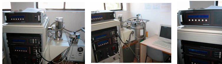
Figure 1. Dynamic Electric Analysis (DEA) equipment used with the control unit for the parameters of the test.
