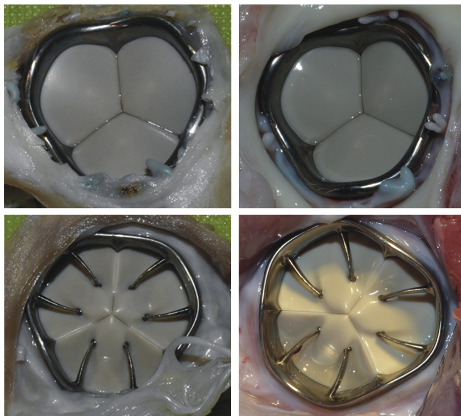
FIGURE 5. Macroscopic aortic ( upper ) and ventricular view of the explanted novel mechanical trileaflet heart valve ( lower ) ( left column , sheep #71270; right column , sheep #81030) after 407 and 375 days, respectively.
