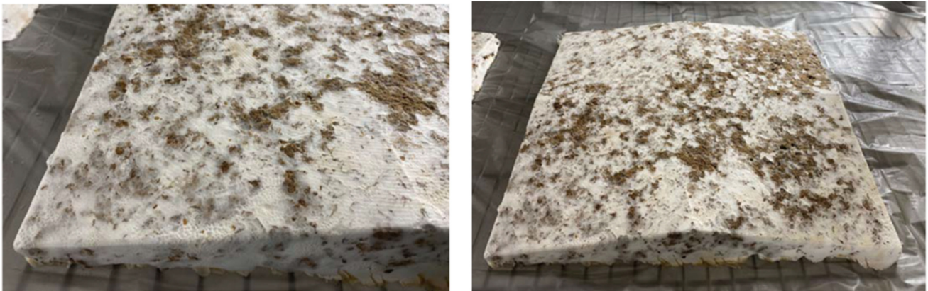
Figure 13. Acoustic panel prototype cultivated with Fine Cardboard substrate.
