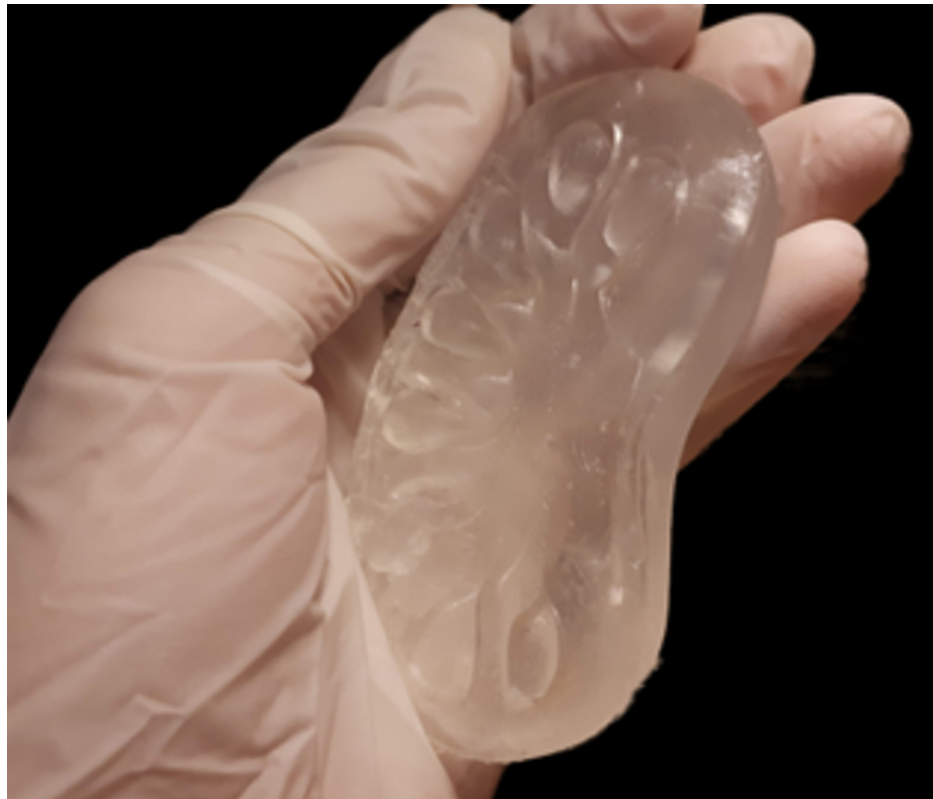
FIGURE 8: Kidney model based on 3D printing and hydrogel
