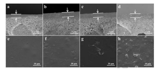
**Figure 6.** SEM cross-section images of (a) pure NaAlg on PAN substrate; (b) (c) and (d) MMMs containing g-C<sub>3</sub>N<sub>4</sub> content 2, 3 and 5 wt% with respect to NaAlg. (e–h) Corresponding surface images of (a) to (d), respectively. Reproduced with permission from [51], published by Elsevier, 2015.
