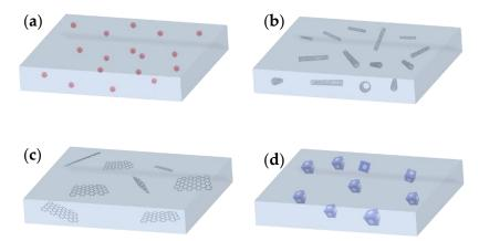
**Figure 1.** MMMs with different dimensional nanofillers; (a) zero-dimensional nanomaterial filled MMM (nanoparticles); (b) one-dimensional nanomaterial filled MMM (carbon nanotube for example); (c) two-dimensional nanomaterial filled MMM (graphene oxide nanosheet for example); (d) three-dimensional nanomaterial filled MMM (microporous nanomaterials).
