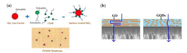
**Figure 2.** (a) Surface modification of silica NPs and the PTMSP/silica MMM. Reproduced with permission from [40], published by MDPI, 2011. (b) Comparison between permeation of GO filled MMM and GOQDs filled MMM. Reproduced with permission from [43], published by Elsevier, 2018.
