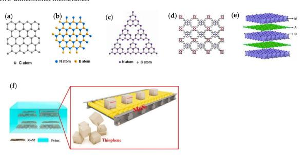
**Figure 4.** Structures of (**a**) graphene, and (**b**) hexagonal boron nitride, (**c**) s-triazine structure models of g- $C_3N_4$ , (**d**) MOF nanosheet and (**e**) layered double hydroxides. Reproduced with permission from [71], published by American Chemical Society, 2017. (**f**) MoS<sub>2</sub> in Pebax as transport facilitator for thiophene. Reproduced with permission from [52], published by Elsevier, 2018.
