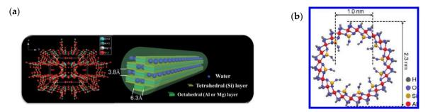
**Figure 3.** (a) Structure of attapulgite nanorod. Reproduced with permission from [46], published by Royal Society of Chemistry, 2016. (b) Aluminosilicate single-walled nanotube. Reproduced with permission from [48], published by American Chemical Society, 2012.
