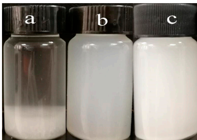
Figure 2. Appearance of bagasse fibers and two nanocelluloses: (a) Dispersion of bagasse fibers; (b) Suspension of CNCs; (c) Suspension of CNFs.
