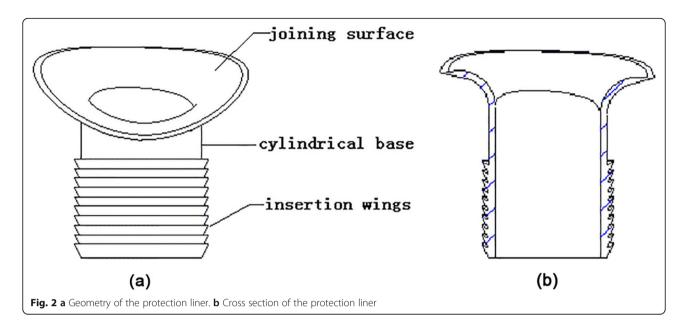
the sharp bone tunnel entrances would first be rounded using a bone drill, then the protection liner would be inserted into the bone tunnels. The cylindrical base would be completely inserted into the bone tunnel and the trumpet-shaped surface would cover the tunnel entrance.
