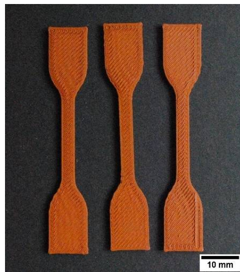
Figure 9. Tensile bar produced with F2_ST filaments at a temperature of 200 °C.
