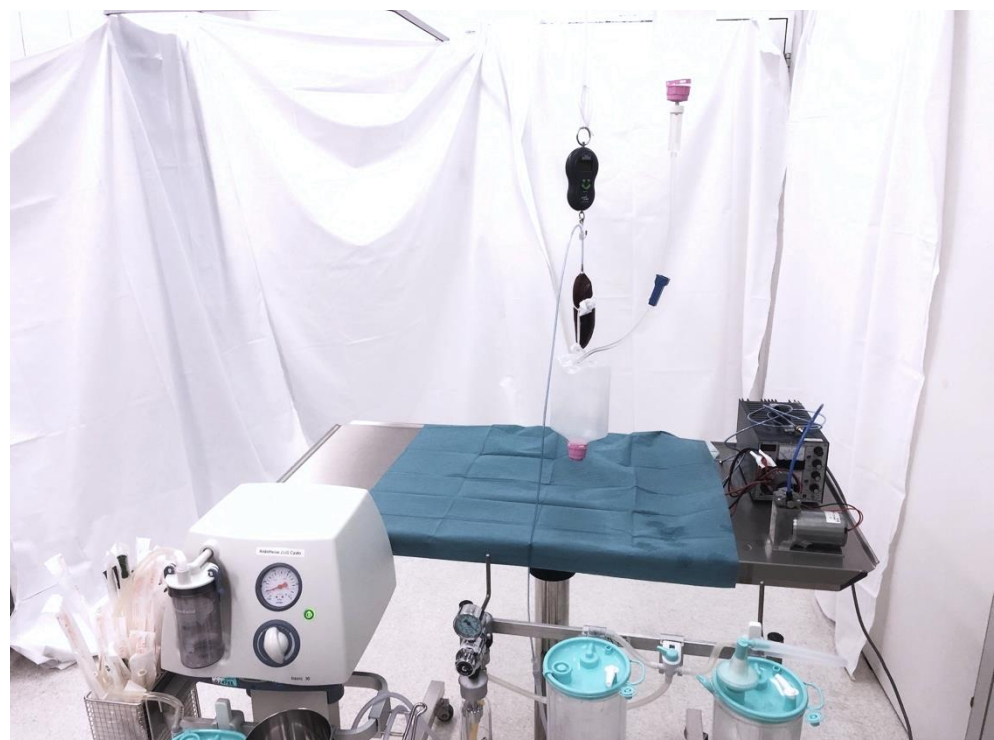
Figure 3. Setup of the holding experiments. The kidney was serially connected with a digital spring balance, completely uplifted, and exposed to additional weight by continuously filling the infusion container attached to the kidney. Negative pressure was provided by a standard OR vacuum suction device.
