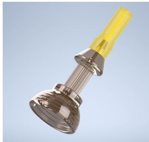
Figure 1. Prototype #2 of THD produced with stainless steel. The conical end is dome shaped for optimal contact with the tissue, the upper pole is designed to firmly connect with a hose. The inner bore at the level of the hose connection was widened to 1.8 mm, and the retention grid was removed.
