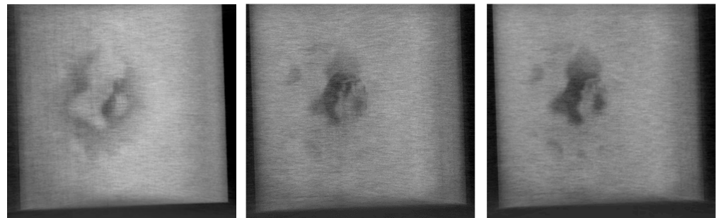
Figure 17. Glare specimen with nonuniform resin regions.
