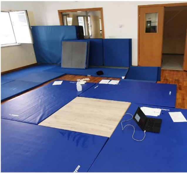
Fig. 4. Data collection set-up: The smart floor is the white square surface surrounded by landing mats. It differs from Fig. 3, because covered with the laminate layer. Notice the laptop linked to the smart floor for data acquisition.
