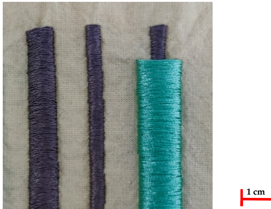
Figure 1. The embroidered conductive-thread patches in the two variations, with the control pattern on the left-hand side.
