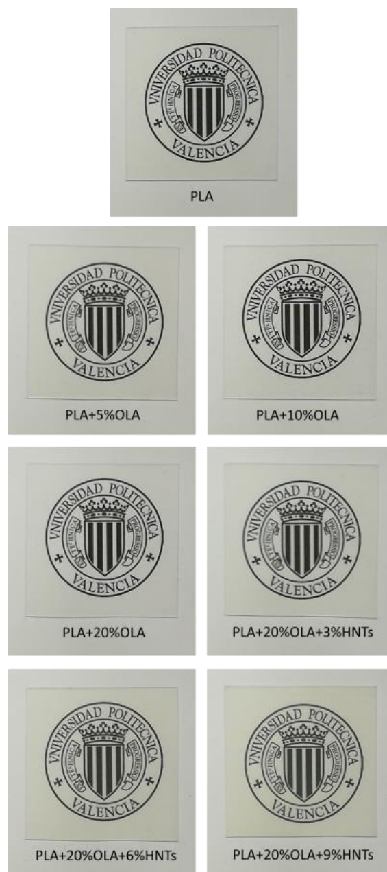
Figure 1. Visual aspect of the polylactide (PLA)/oligomer of lactic acid (OLA)/halloysite nanotubes (HNTs) films.
